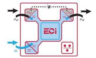
The ECI technology eliminates all single points of failure with full scalability; up to 32 modules in parallel and high efficiency of up to 96% in AC to AC conversion, and above 94.5% in DC/AC conversion, hence reducing operating costs.
